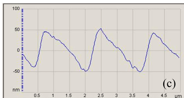
FIG. 1. (Color online) (a) Photo of resist master grating. The measured metrological box is shown with circle. (b) 3D reconstruction of AFM image of measured box. (c) Example of AFM profile of measured metrological box.
